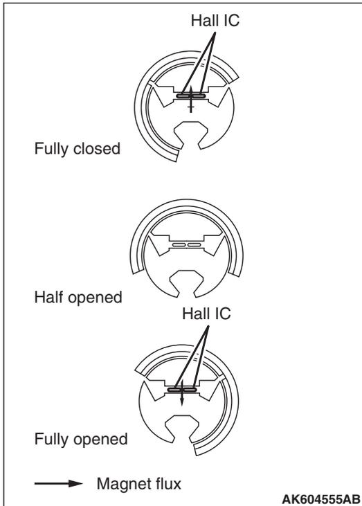
Magnetic flux density at Hall IC is proportional to the output voltage.
