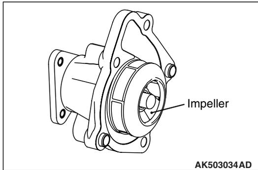
The water pump is the centrifugal, impeller type that is installed in front of the cylinder block. It is driven by the drive belt.
