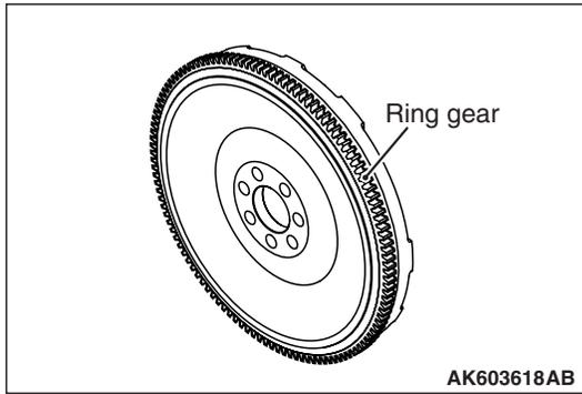
A cast iron ring gear is a shrink fit in the iron casting of the flywheel.
