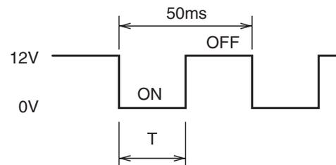
The longer the ON position, the more advanced the intake camshaft angle
