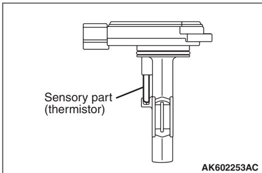
Intake air temperature sensor is built in to the mass airflow sensor. Intake air temperature sensor detects intake air temperature through thermistor's resistance change and outputs the voltage according to intake air temperature to ECM. ECM uses this output voltage to compensate fuel injection control and ignition timing control. Sensor properties are as shown in the figure.
