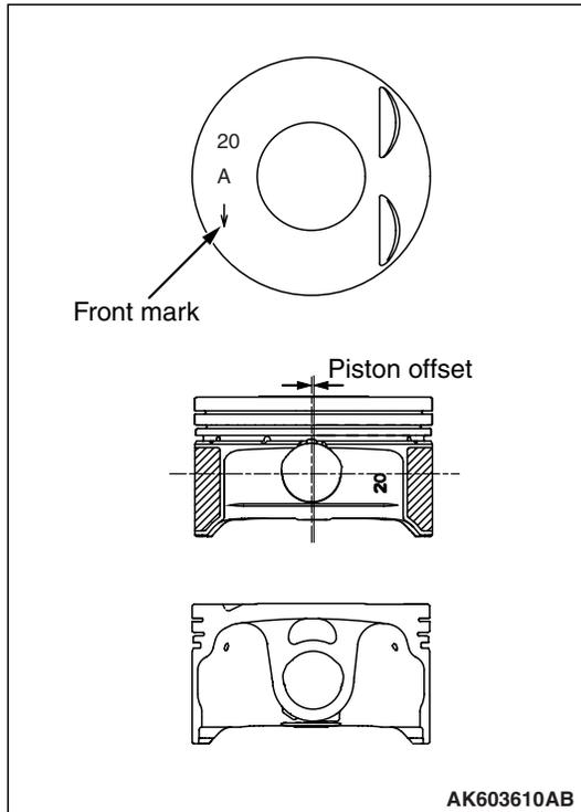
The pistons are made of a special aluminum alloy. Their weight has been reduced by lowering their overall height and increasing the depression at each end of the piston pin. The piston pin hole center is offset 0.8 mm (0.031 in) towards the thrust side of the piston center. The skirt portion along the perimeter of the piston is finished with streaks that excel in oil retention and seizure resistance.
