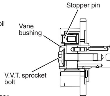
Exhaust V.V.T. sprocket
