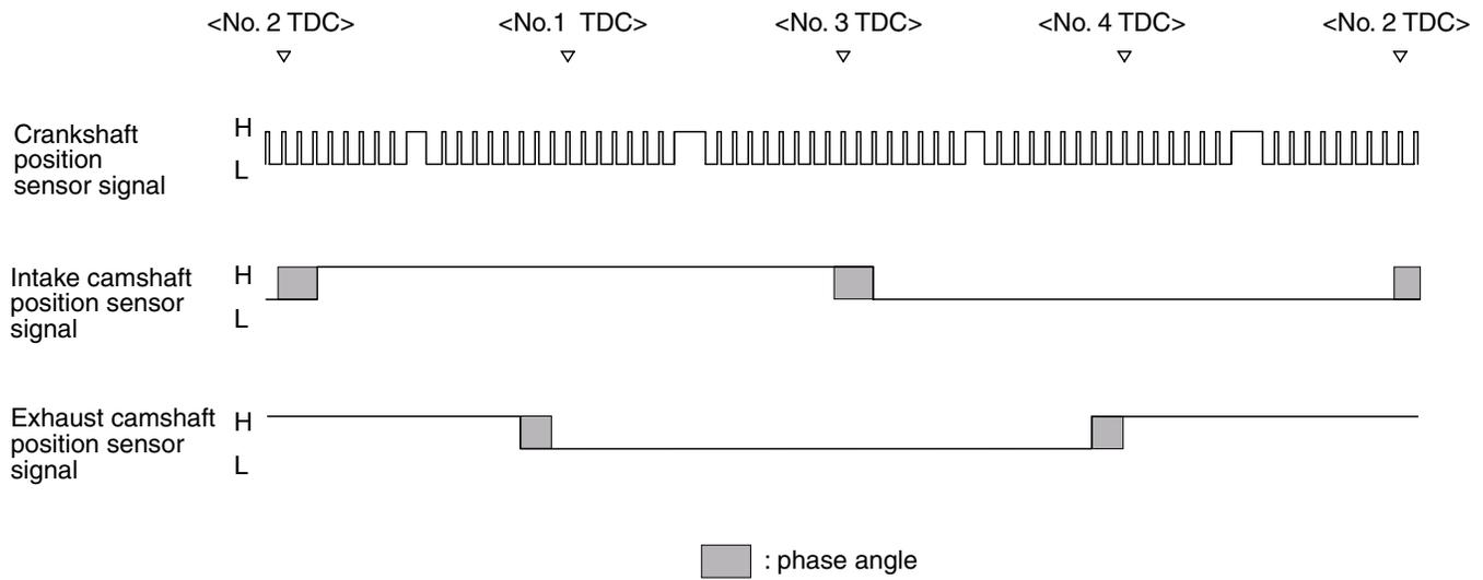
The detected phase angle is calculated using the cam position sensor signal.
