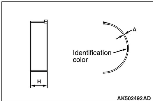
The upper and lower connecting rod bearings are the same. Each connecting rod bearing is provided with a backing plate. Its bearing portion is made of an aluminum alloy and its backing plate is made of ordinary sheet steel.
