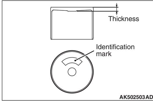
To adjust the valve lift, 47 sizes of valve tappets are available in 0.015 mm (0.0006 in) increments, from 3.000 mm (0.1181 inch) to 3.690 mm (0.1453 in).
