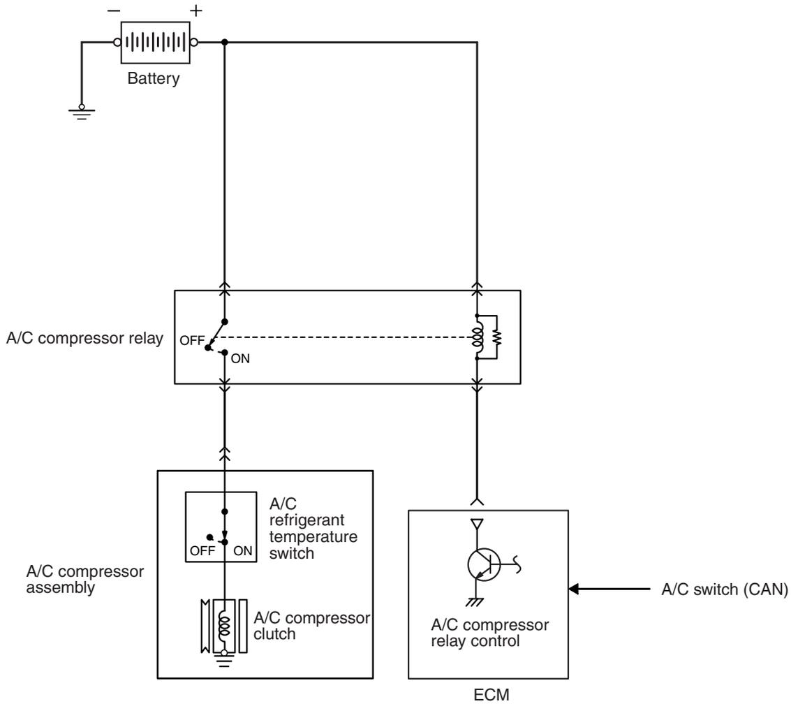
The ECM turns on the power transistor when the A/C switch ON signal is input by the A/C-ECU through the CAN. This allows the A/C compressor relay to be ON and to be operated. During the high load operation, such as the acceleration with the fully opened accelerator, the ECM secures the acceleration capability by turning off the A/C compressor relay for the specified period to produce no load on the A/C compressor.
