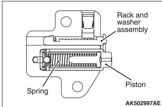
The tensioner maintains the tension of the timing chain. It contains a piston with a built-in spring. With the tensioner installed, its piston directly pushes on the tension lever in order to automatically adjust the tension of the timing chain.
