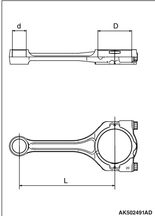
The connecting rods are made of highly rigid, forged carbon steel. The cross section of the rod portion is shaped like the letter H.
