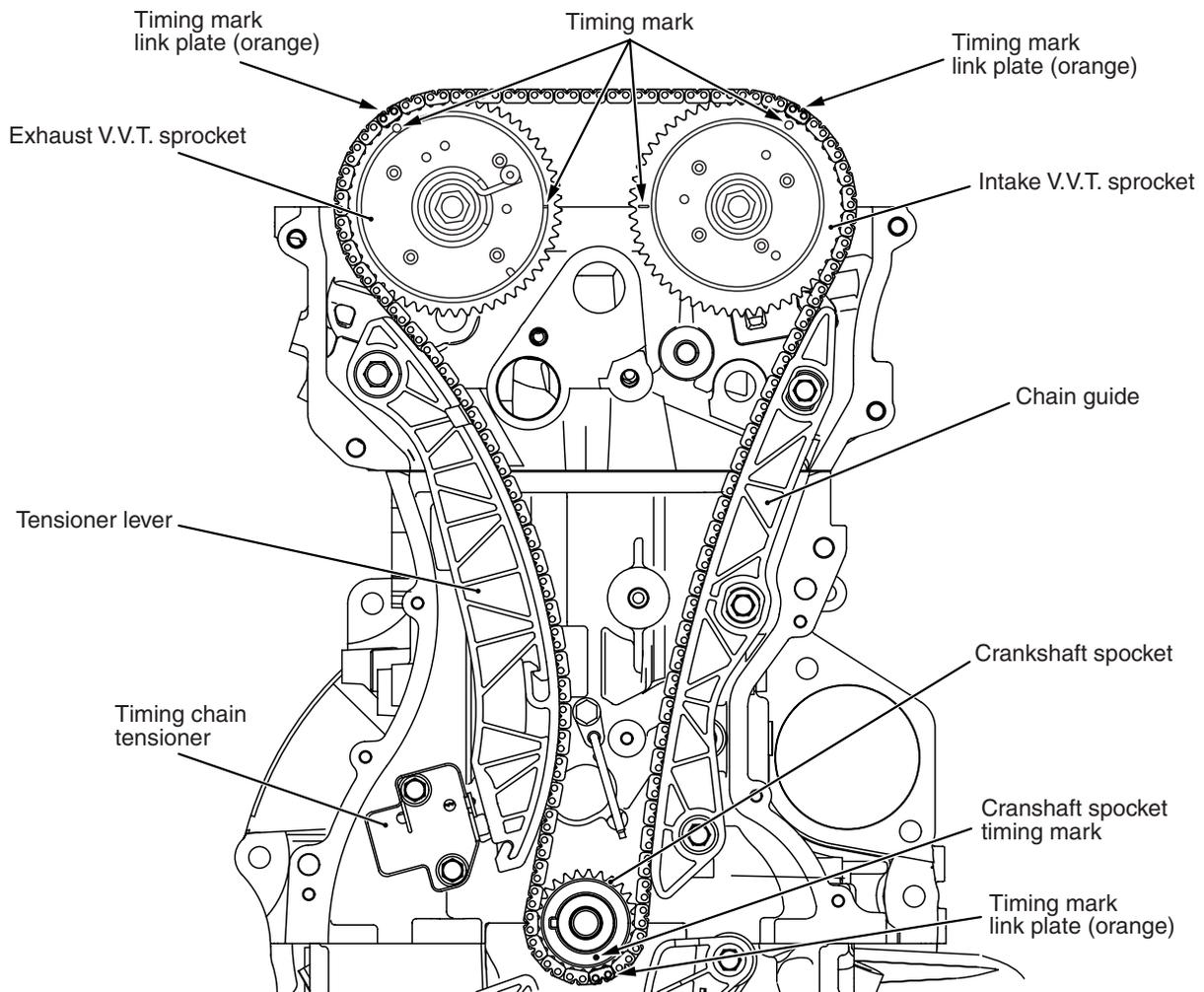
The two camshafts are driven by the timing chain via the camshaft sprockets.
