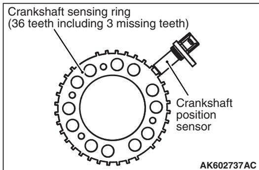
A crankshaft position sensor is installed on the right side of the cylinder block. The crankshaft position sensor monitors rotation of crankshaft sensing ring (36 teeth including 3 missing teeth) installed on the crankshaft and converts to voltage (pulse signal) that is output to ECM. ECM uses crankshaft position sensor's output pulse to detect crankshaft position.
