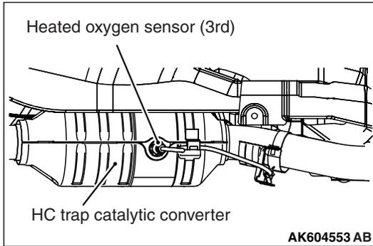
The heated oxygen sensor (3rd) is installed to the HC trap catalytic converter. The heated oxygen sensor (3rd) detects the oxygen density of the exhaust gas and outputs the voltage to the ECM in accordance with the oxygen density. The ECM uses this output voltage to detect the deterioration of the HC trap catalytic converter. The structure of the heated oxygen sensor (3rd) is the same as that of the heated oxygen sensor (rear) installed in the exhaust pipe.
