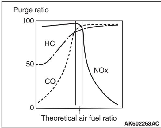
This allows ECM precise feedback control to get theoretical air-fuel ratio with best cleaning efficiency of 3-way catalytic converter.
