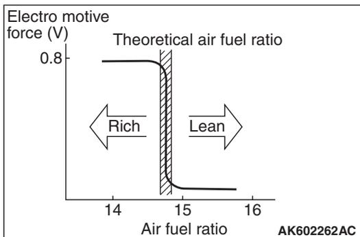
This sensor uses the oxygen concentration cell principle of solid electrolyte (zirconia) and displays the property of sudden change in output voltage near theoretical air-fuel ratio. This property is used to detect oxygen density in exhaust gas. Feedback to ECM allows it to judge whether air-fuel ratio is rich or lean compared to theoretical air-fuel ratio.
