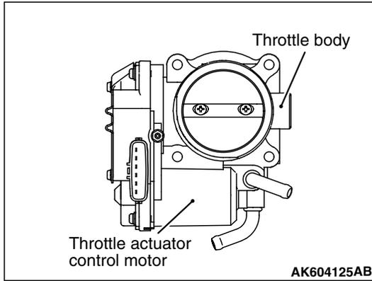
A throttle actuator control motor is installed in throttle body. The throttle actuator control motor performs the Open/Close of the throttle valve through the reduction gear. ECM changes current direction according to the Open/Close direction and also changes current to the motor coil to control the throttle actuator control motor.
