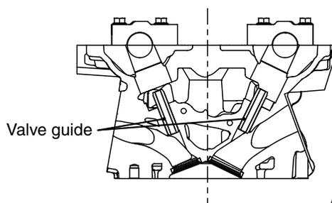
A cylinder head made of an aluminum alloy, which is lightweight and offers a high level of cooling efficiency, has been adopted. A pentroof combustion chamber with a center spark plug has been adopted. It has a small valve compound angle to realize a compact chamber.
