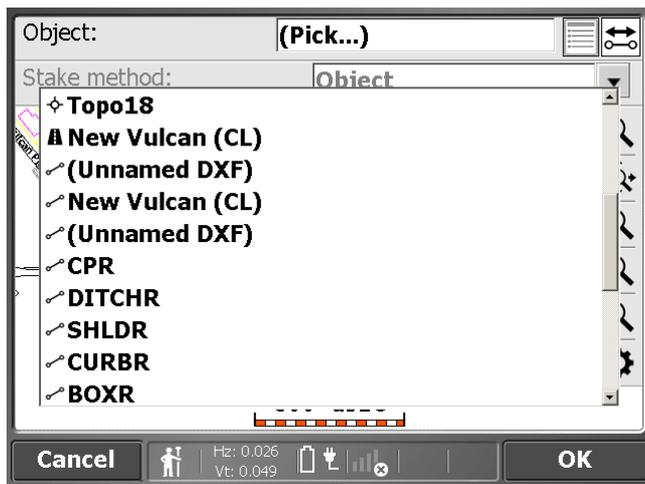
3. If necessary, before confirming the selection, change the line direction using the button on the top right of the screen.
